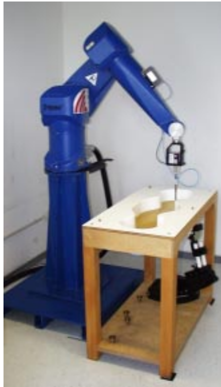
Fig. 2: The measurement setup with a phantom containing tissue simulating liquid and a device under test.
